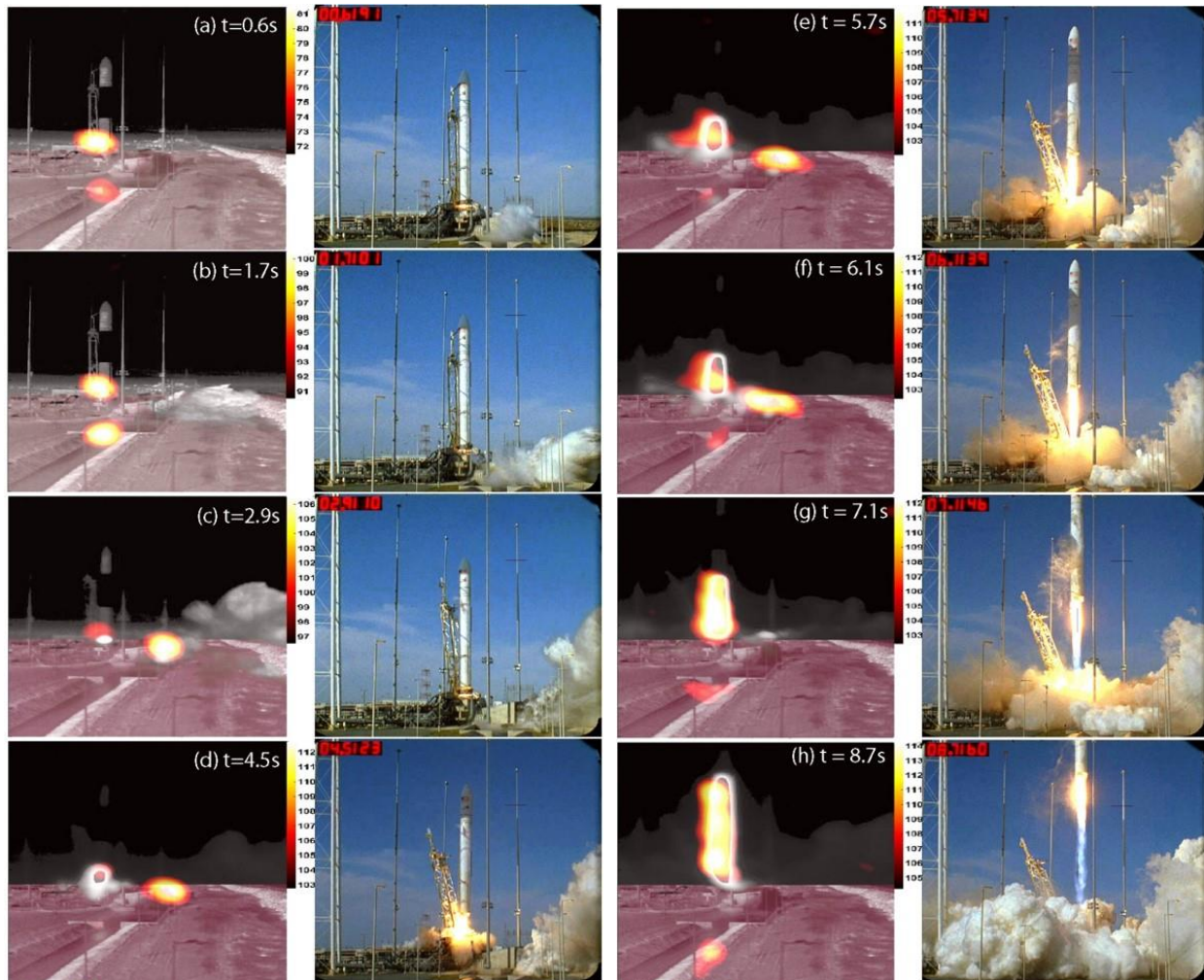
Figure 11. Left column noise maps superimposed on frames from IR camera, conventional beamform at 2kHz; (right) corresponding frames from a high-speed camera. (Reproduced from Fig. 11, Ref. 26).
